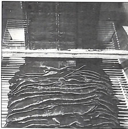
The wool seen through a window and heaped on the conveyor of the steamer with the cover removed
