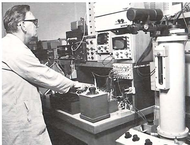
The calculable capacitor used as a basis for electric impedance standards.
