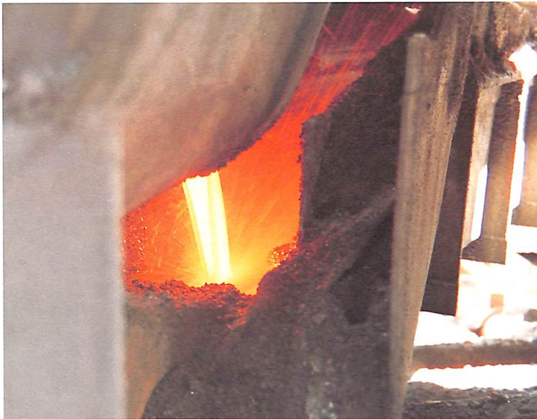
High intensity smelting by Siros melt technology: molten high-lead slag being tapped from the Mount Isa Mines pilot plant for direct smelting of lead concentrates. This version of the process is known as ISASMELT.
