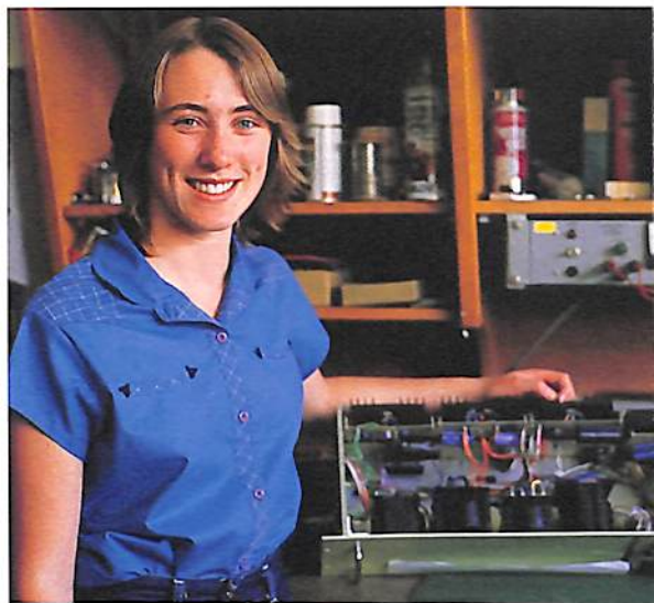
Elizabeth Fowle (apprentice technician) with the power supply unit for the CSIRO Parkes Telescope's new Q band (42 to 50 GHz) receiver. The unit was built by Elizabeth to specifications provided by Graham Gay (senior technical officer).
