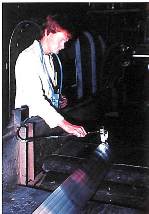
A scientist from the Division of Applied Physics working on the development of a ratio pyrometer for temperature measurement in an aluminium strip rolling mill.
