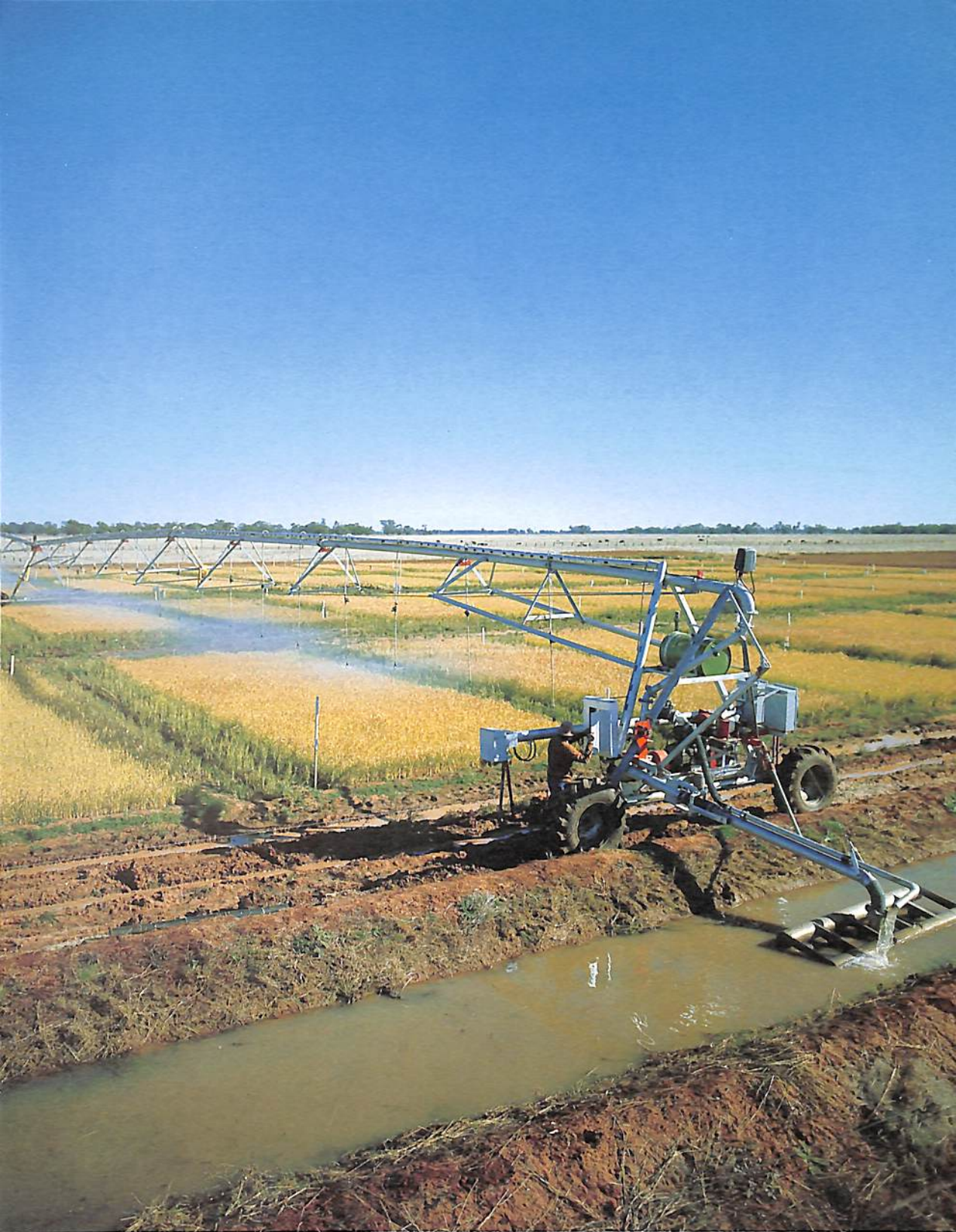
A lateral move irrigator traverses the field automatically and applies a predetermined volume of water to experimental plots by overhead spray. Adjustments enable different rates to be applied to different plots in one pass.
