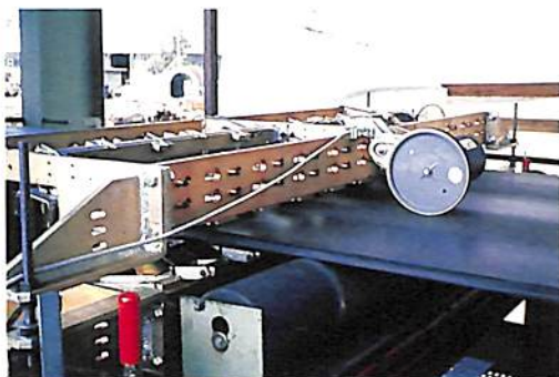
The Division of Applied Physics developed this conveyor belt monitor to detect flaws. It is finding good markets in Australia and overseas.
