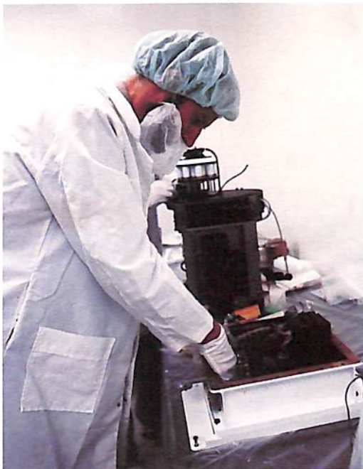
Mr Peter Osman, of the Division of Applied Physics, works the CSIRO instrument carried aboard a NASA space shuttle. It was designed to measure the viscosity of normal and diseased blood under the zero gravity conditions of space. It is hoped the results will lead to a better understanding of blood clotting.
