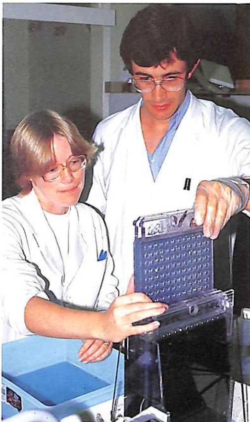
Protein fractionation, using electrophoretic techniques, allows the genetic origins of food materials to be identified quickly. The process was developed by the Wheat Research Unit.
