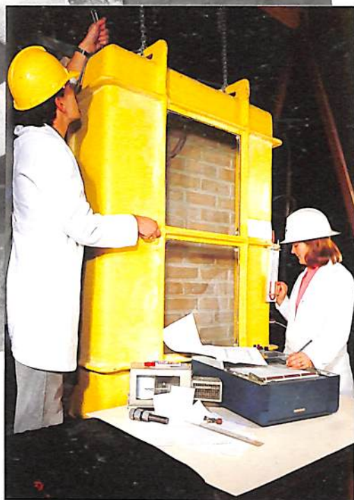
Small wall sections mounted in a test rig are subjected to simulated rain and wind pressures as part of the 5-Star Design Rating project. Filling the cavity between internal and external skins of walls could improve the energy efficiency of buildings; it could also increase the potential for water to penetrate the walls.
