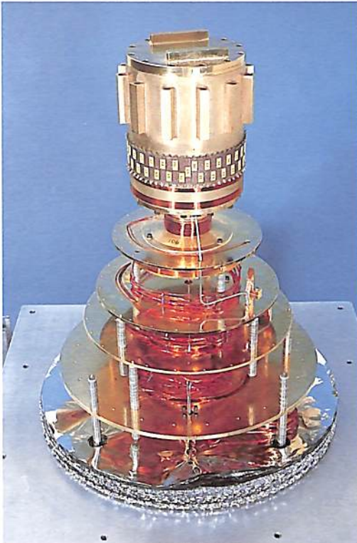
The main assembly of the gas thermometer used to establish part of the international thermodynamic temperature scale.
