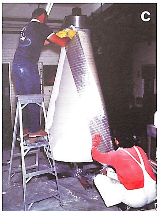
One of the new low-cost, lightweight Australia Telescope horns for L/S bands (1.25 to 2.5 GHz), 1 m wide at the aperture and 2 m long. Bands of aluminium (a) surrounding polystyrene foam discs are stacked to form the shape required (b). Sheets of fibreglass are bonded on (c) — by a professional boat builder — and with its finished coat of epoxy resin the horn is ready for testing (d).
