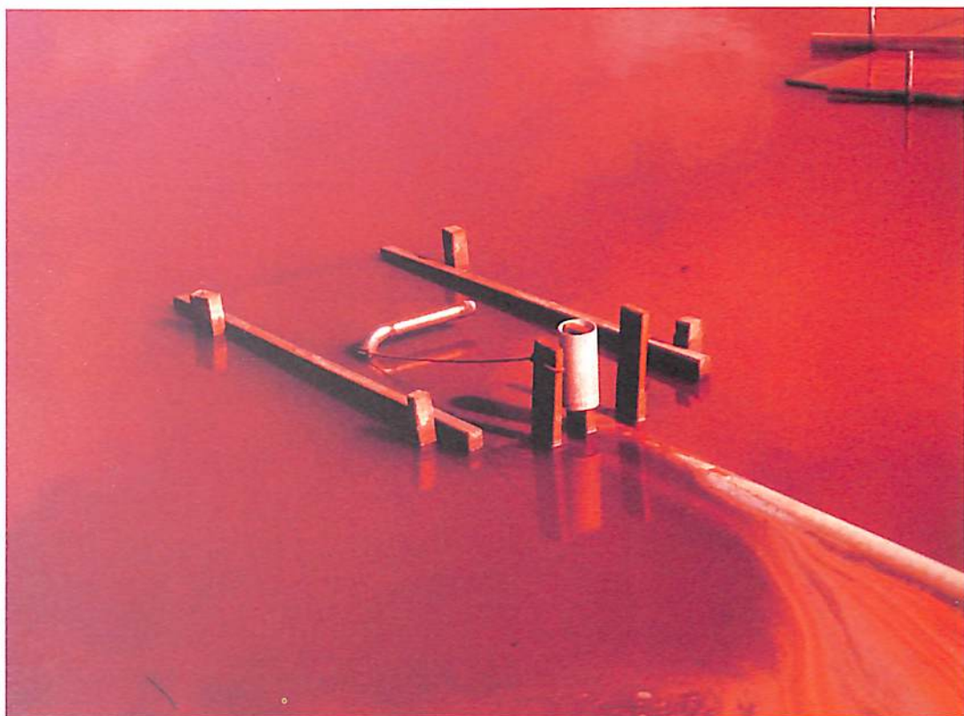
Pumping Dunaliella salina , the source of beta-carotene, to the Whyalla plant from this brine culture pond.
