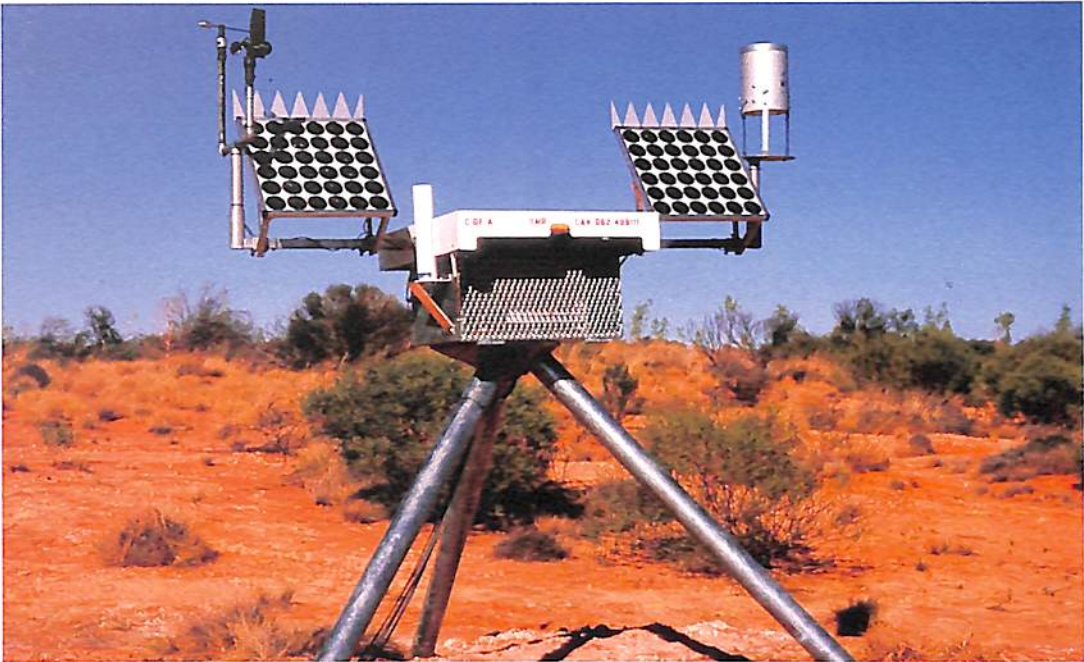
A solar-powered data acquisition platform used in remote locations.
