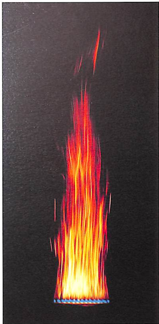
Fine particles of Milmerran coal burning in a laboratory-scale gas-stabilised flame, during studies of ignition and ash formation.
