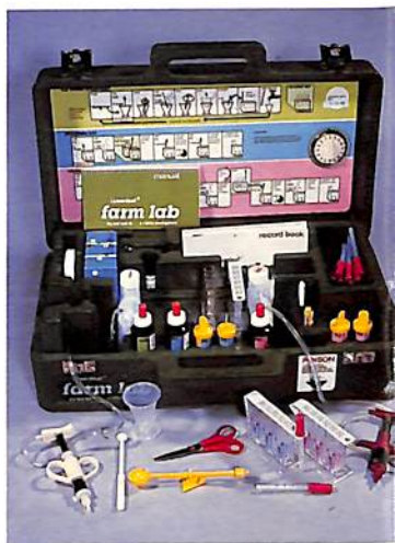
The GREENLEAF FARMLAB kit analyses plant tissue quickly and simply, helping farmers check for nutrient shortages in growing crops and pastures.
