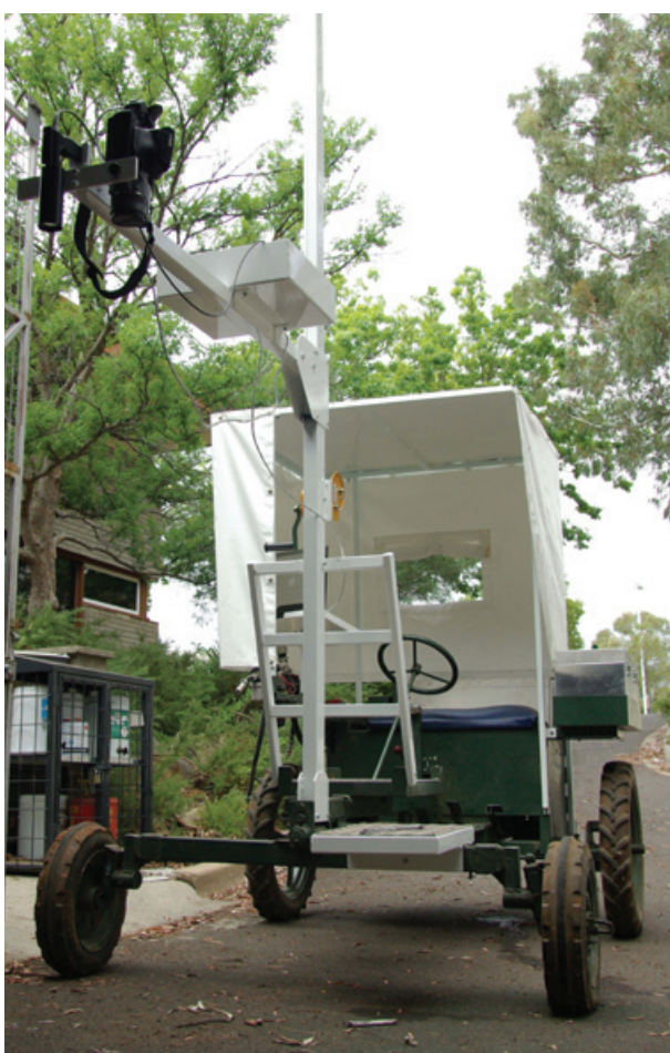
The 'phenomobile' was designed and developed by the HRPPC to integrate a range of remote sensing technologies for phenomics field studies
