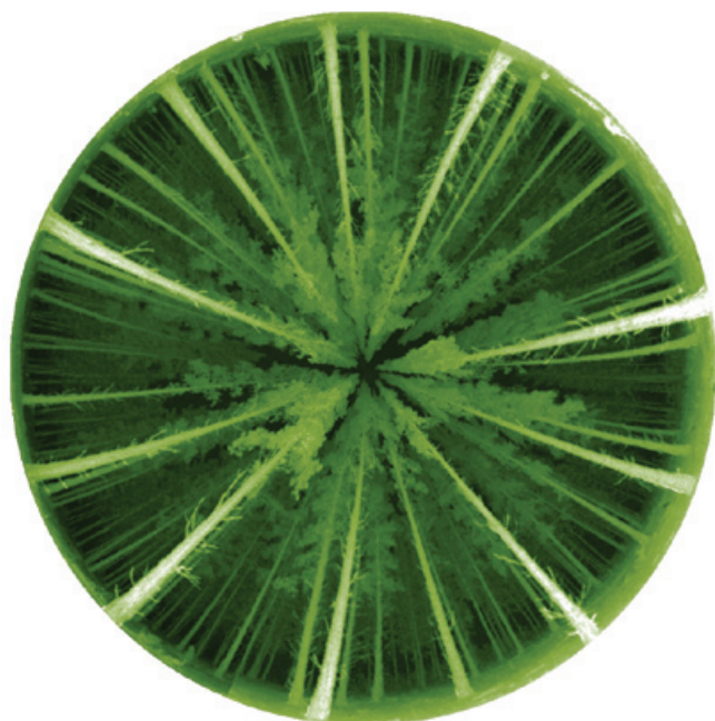
Simple 2D projection of ECHIDNA Validation Instrument (EVI) cumulative waveform intensity mature Pinus radiata
