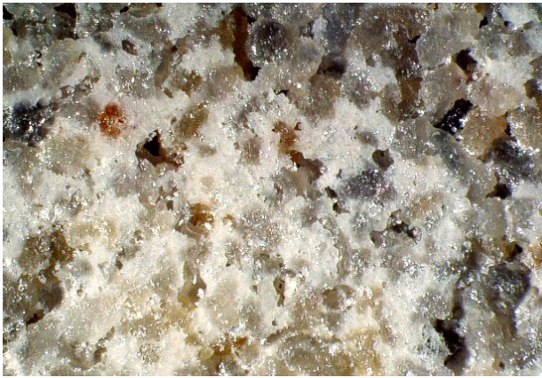
1-2mm sand grains (grey, yellow and brown) heavily encrusted with CIPS calcite (white).
