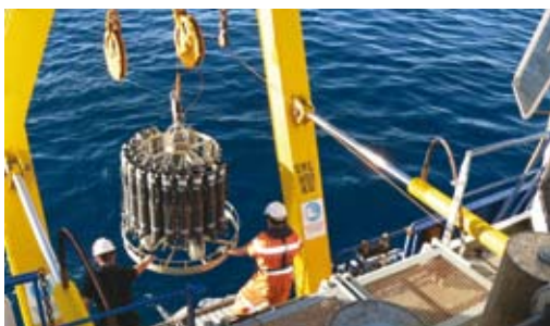
Deploying an instrument designed to monitor the distribution and variation of water temperature, salinity, and density. It was used to collect water samples at specific depths. Photo: Bob Beattie
