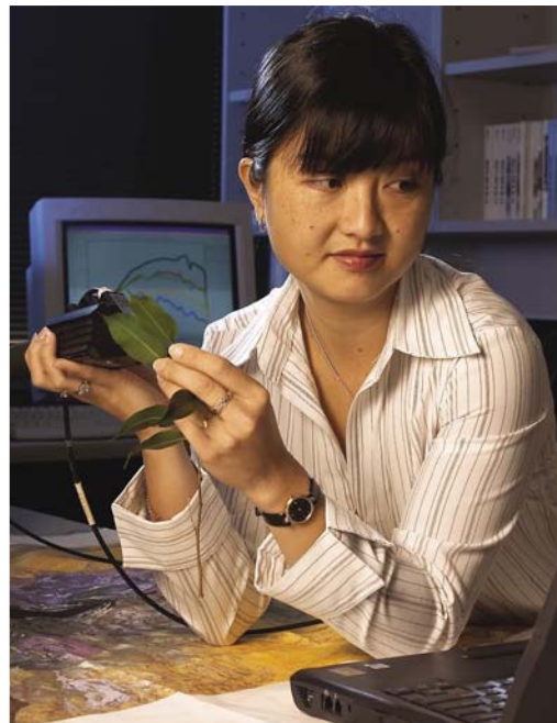
Cindy Ong examines leaves and rock samples from the Goldsworthy mine with a field spectrometer to help generate environmental measurements from the site. Photo: Kevin Scott, SKS Corporate Photographers
