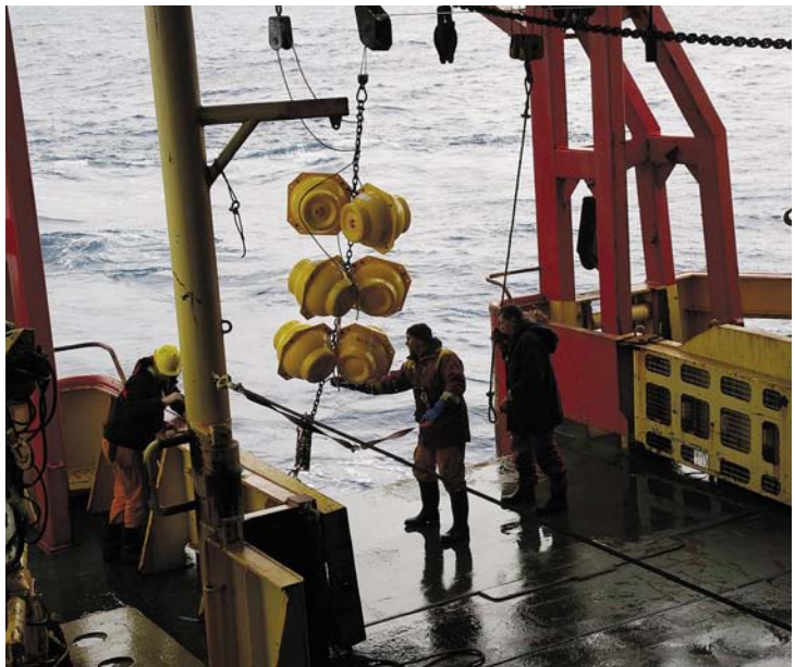
Crew retrieve moorings from the Antarctic resupply vessel, Aurora Australis , in January 2005. Mooring instruments record ocean conditions from the sea floor to the surface. Photo: CSIRO
