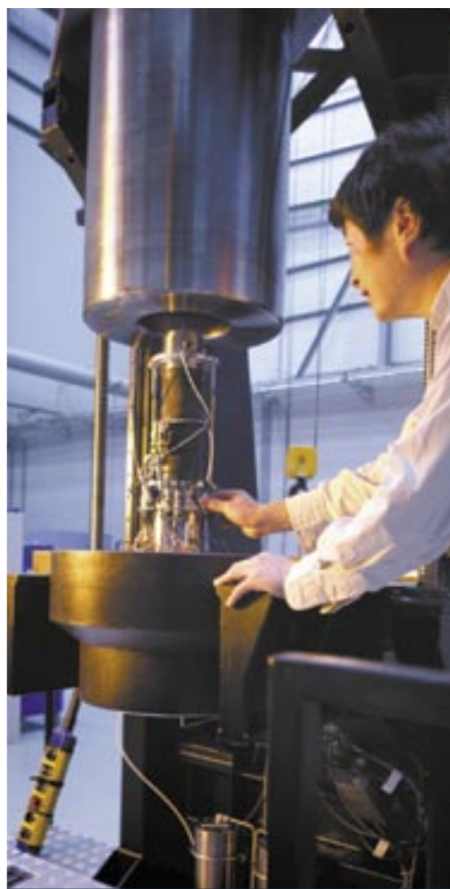
A thick-walled hollow cylinder sample is being setup in the high pressure triaxial cell to study wellbore instability mechanisms and drilling fluid and shale interaction. Photo: CSIRO
