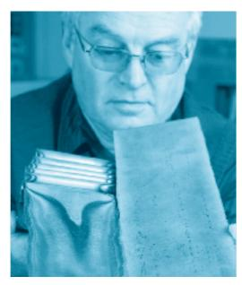
Nigel Stone with early samples from trials of a new process to continuously manufacture titanium sheet from powder. Photo: Mark Fergus
