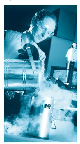
CSIRO's Peter Eadington preparing laboratory equipment to make low temperature measurements on fluid inclusions. Photo: Murray Armenti, Visions Photography
