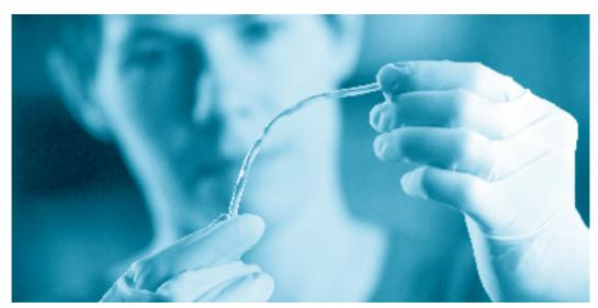
CSIRO's catheter is barely three millimetres in diameter and contains a series of optical-fibre pressure sensors, which measure the waves of pressure when the patient swallows. Photo: David McClenaghan
