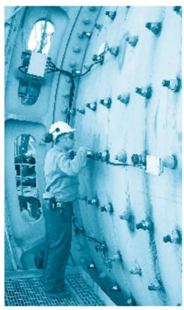
Listening in: Kevin Davey installing accelerometer modules on a production-scale SAG mill. Photo: David Barker
