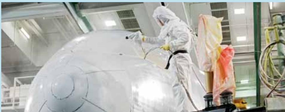
CSIRO-Boeing's 'spray on and leave on' paint being applied to an aircraft. Credit: CSIRO
