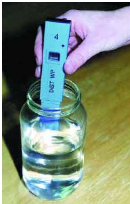
Figure 2. Measuring electrical conductivity with a hand-held meter.
