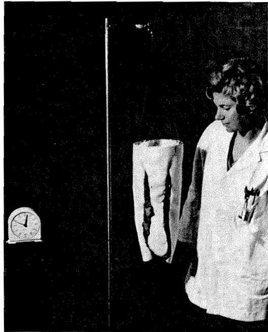
Above: Wool material shaped to simulate a child's skirt. It took 15 seconds to ignite in the test, and after burning in two small vertical strips, extinguished itself in two minutes.
