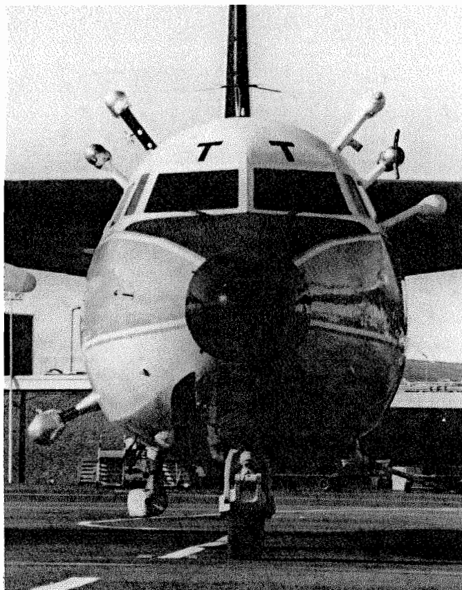
Bristling with scientific equipment, CSIRO's specially modified Fokker F-27 is used for a variety of projects, from trapping atmospheric particles to bouncing beams off land and sea.
