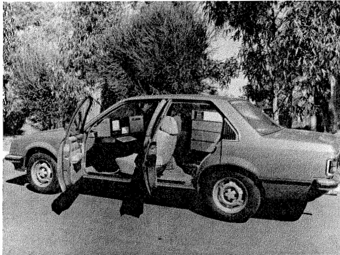
The test car that Dr Johnston's team uses has a microcomputer system that continuously records 14 variables concerned with the car's operation. These include fuel flow and temperature, acceleration, engine rpm and engine oil and coolant temperatures.
