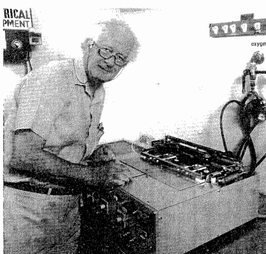
Keith Norrish and an x-ray spectrometer; fast testing of ore composition means significant savings in shipping costs
