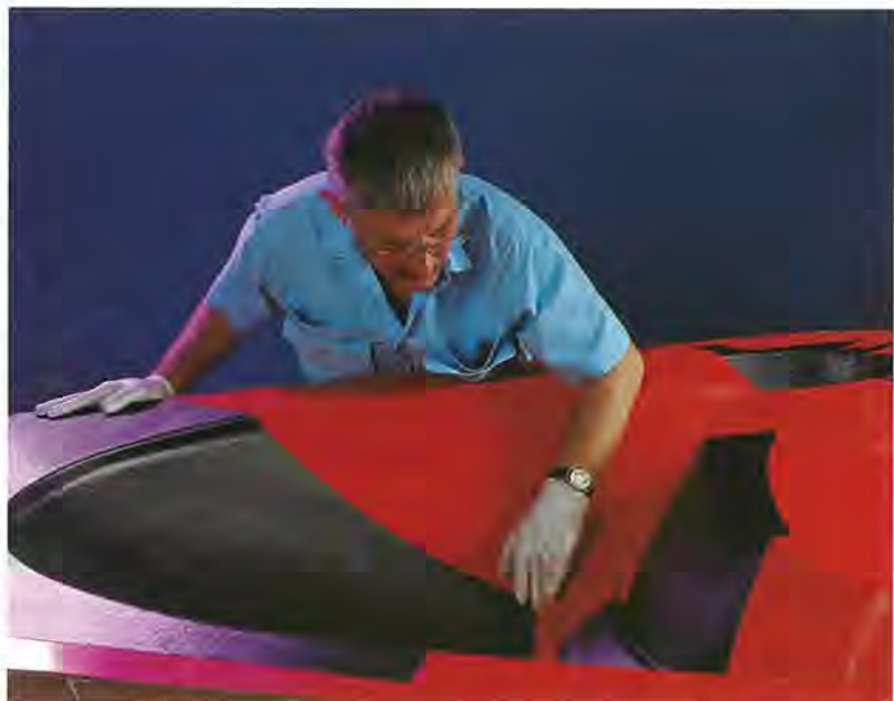
Placing composite materials in a mould.
