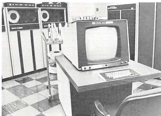
Cyber 730 operator station: the computer can be controlled from this interactive terminal. In the background are some of the 9-track tape drive units connected to the Cyber 730.
