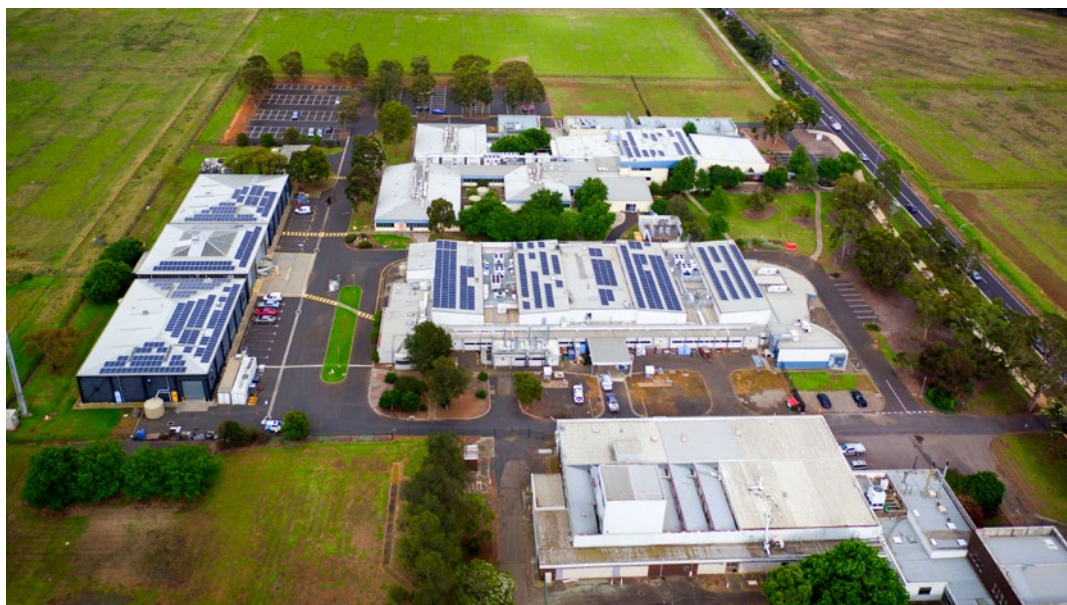
The 300-kilowatt solar photovoltaic system at our Werribee site comprises 1,000 solar panels.
